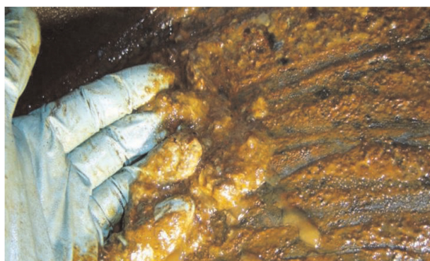
Figure 3. Sludge formed from lubricating oil. Reprinted from Livingstone et al. (2007) .
